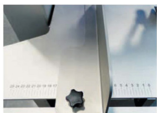
Scala graduata sul piano di lavoro Worktop with graduated scale
